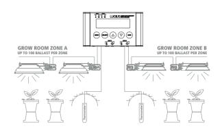
4 Connect the Temperature Probes to the Lucius LMC socket. There are 2 Temperature Probes each for the use in its own zone.
