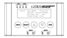
Press button to go to the next menu. The forth menu is "Data Display" in this menu it displays all data. You also can adjust the power manually by using button (A), and (V).
