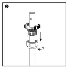
3. Loosen the screw cap on the adjustment knob, let the aluminium tube pass through the screw cap and put into the adjustment knob. Adjust the the desired position and tighten the screw.
