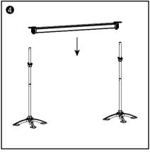
4. Install the light bars by locking the holes on its both sides with the stands.
