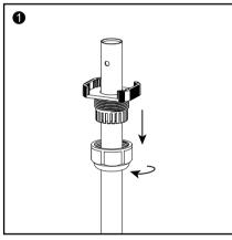
1. Users can prepare two tubes for ICL-300 installation by themselves. Loosen the screw cap on the adjustment knob, let the tubes pass through the screw cap. Adjust the desired position and tighten the screws.
