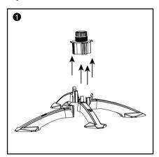
1. Take out the four stand legs of TSD-1, lock the suspension rack with the legs.
