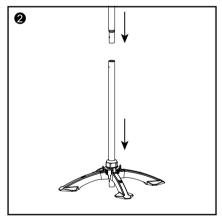
2. Loosen the screw cap, let the aluminium tube pass through the screw and put into the suspension rack. Adjust the the desired position and tighten the screw.
